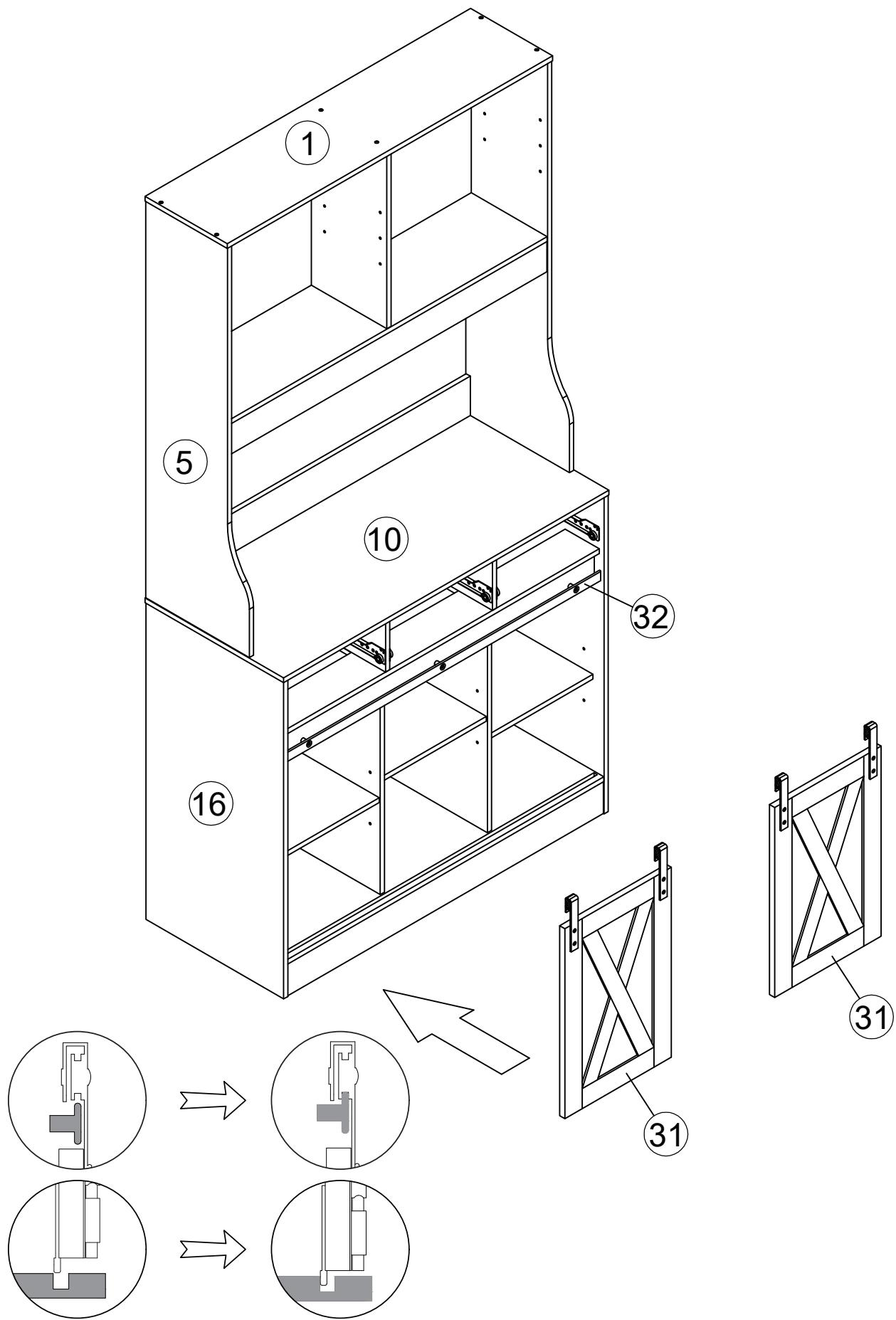
**EN:** The roller is hung on the slide rail, and the "U" component is inserted in to the card slot.
