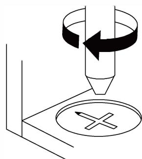
**EN\_Turn cam lock clockwise to tighten.**
