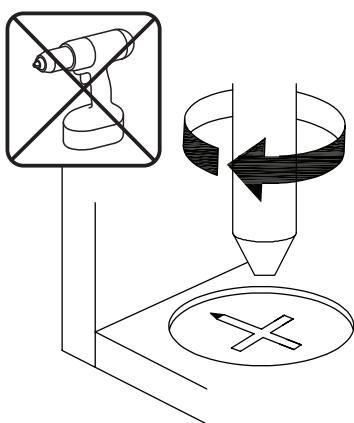
**EN**\_Turn cam lock clockwise to tighten.
