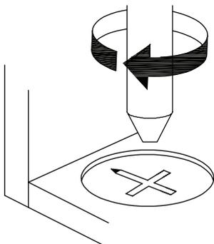
**EN\_**Turn cam lock clockwise to tighten.
